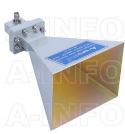
LB-137-15-C-TF Standard Gain Horn Antenna 5.85-8.2GHz 15dB Gain TNC Female
